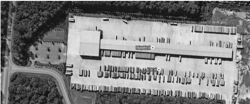
Figure 1.9 Transloading is the transfer of cargo from 20- or 40-foot ocean containers into domestic 48- or 53-foot trailers. Depicted is Pep Boy’s East Coast transload facility located near the Port of Savannah, Georgia.
